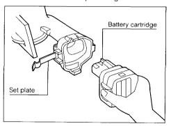
•Do not use force when inserting the battery cartridge. If the cartridge does not slide in easily, it is not being inserted correctly.
